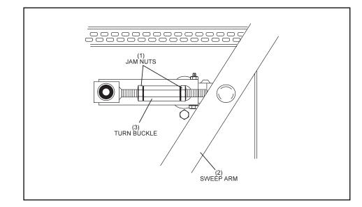
Figure 6-67. Turnbuckle Jam Nuts Viewed from Right Side of Pinsetter.
