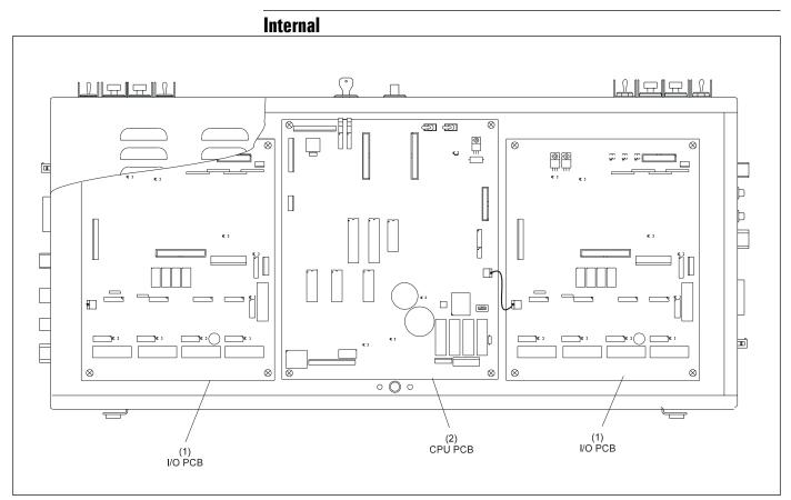
Figure 4-10. Internal View - Consolidated Low Voltage Box.
