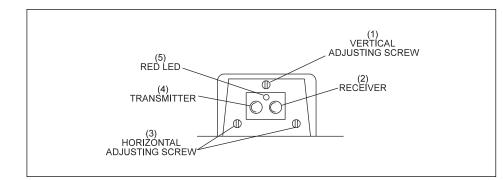
Figure 6-2. Ball Detect Adjusting.
