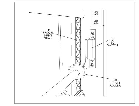
Figure 2-3. Shovel Roller Pulsing EC Switch.
