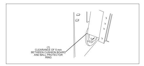
Figure 6-9. 5 mm Clearance Between Cushion Board and Ball Protector Ring.
