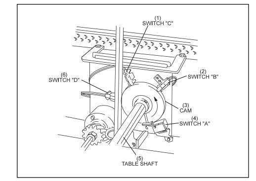
Figure 1-35. Switch Cluster Assembly.
