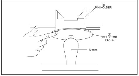
Figure 6-47. Pin Detector Plate Clearance.
