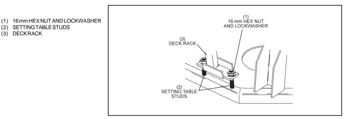
Figure 6-33. Setting Table Studs.
