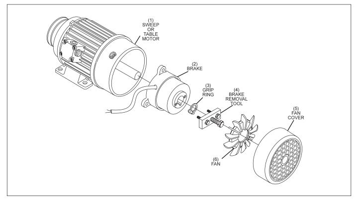
Figure 8-31. Motor Brake Replacement
