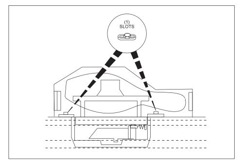
Figure 6-30. Position of Pin Station in Distributor.
