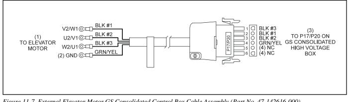
Figure 11-7. External Elevator Motor GS Consolidated Control Box Cable Assembly (Part No. 47-142616-000)
