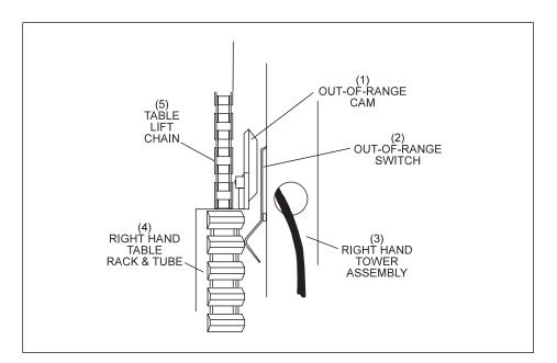
Figure 2-6. Out-Of-Range Switch.
