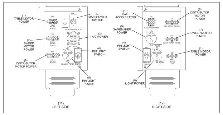
Figure 8-13. Left and Right Side Views - Consolidated High Voltage Box.
