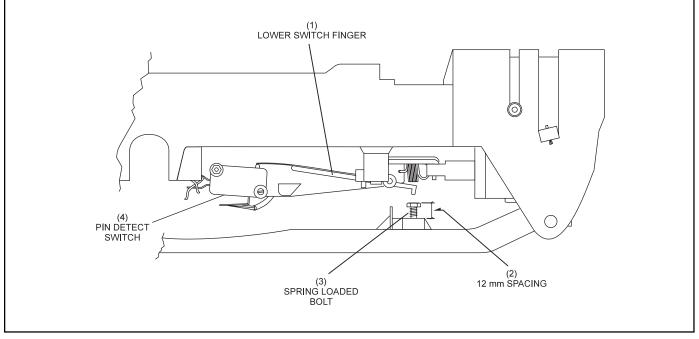
Figure 6-54. Pin Detect Switch Adjustment
