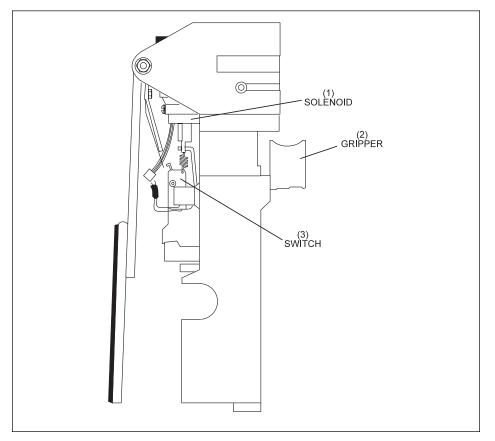
Figure 2-23. Pin Holder Vertical - Setting Pin on Lane.
