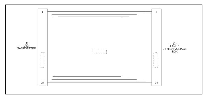
Figure 10-16. Solenoid Data Cable (Part No. 68-100046-000)
