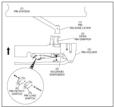
Figure 1-19. Loading Pins.
