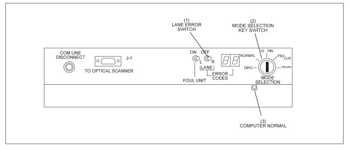
Figure 3-10. Universal Electronics Diagnostics.
