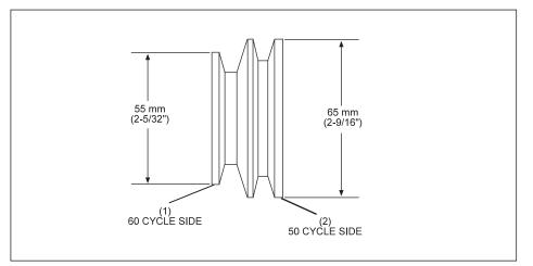
Figure 8-28. Dual Pulley.
