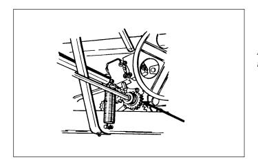
8. Spotting Tong Clutch Gear Cluster A. Grease the 1 or 4 gears lightly.
