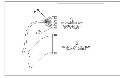
Figure 6-78. Checking +5 Volts on Gamesetter.
