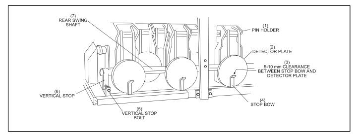
Figure 6-46. Pin Detector Plate's Vertical Adjustment.
