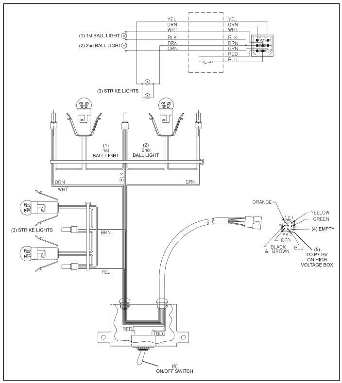
Figure 10-11. Masking Unit Cable (Part No. 53-200871-000)
