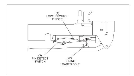
Figure 2-10. Pin Holder Detecting (GS-96 and Early GS-98)
