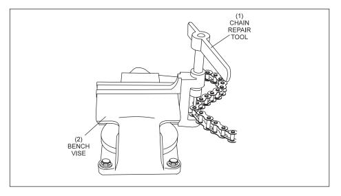
Figure 8-32. Chain Repair Using Vice.
