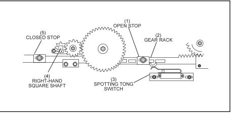
Figure 6-59. Adjustable Stops on Setting Table Tong Rack.
