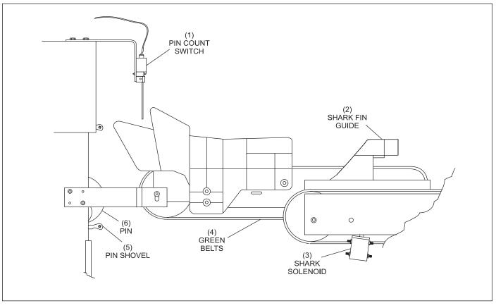
Figure 2-24. Shark Solenoid (GS-96s and Later)
