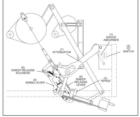
Figure 1-28. Sweep Release - Raised Position.
