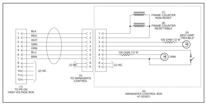
Figure 10-20. Manager's Remote Control Cable (Part No. 68-100159-000)
