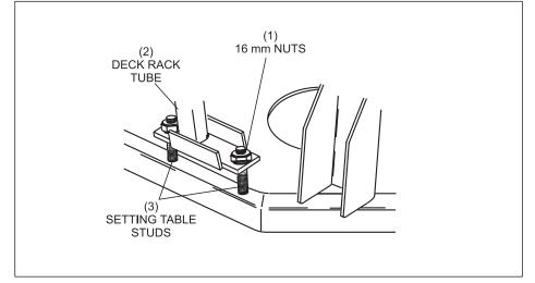
Figure 8-6. Removing Table from Deck Rack Tubes.
