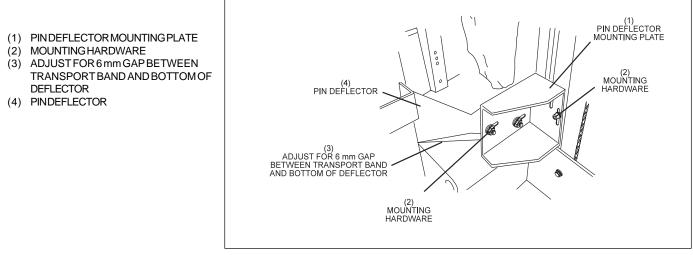
Figure 6-21. Deflector Positioning for Proper Clearance
