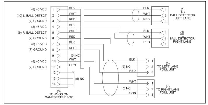
Figure 10-5. Optical Trigger & Foul Cable (Part No. 47-192592-000)
