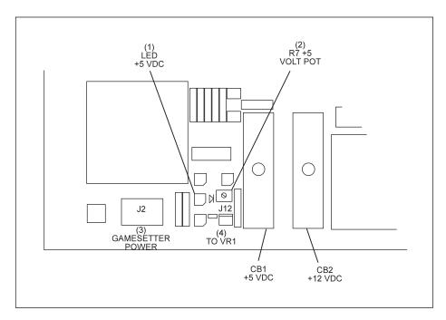
*NOTE:* The 5 volts should be kept as close to +5.14 VDC as possible. *Figure 6-79. Adjusting +5 Volts in Common Box.*
