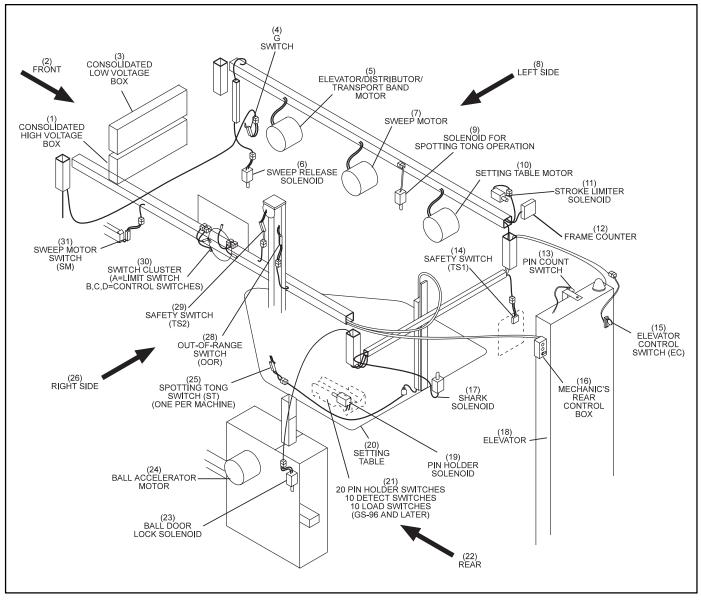
Figure 11-1. GS-98 Pinsetter Electrical System Overview with Consolidated Electronics
