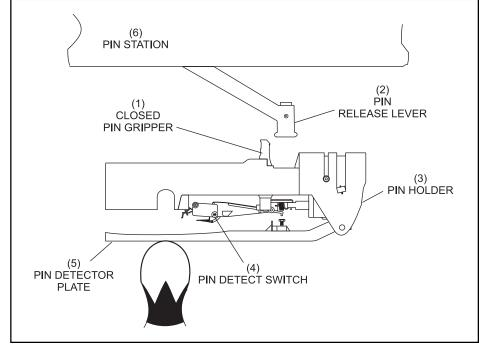
Figure 1-18. Detecting Pins.
