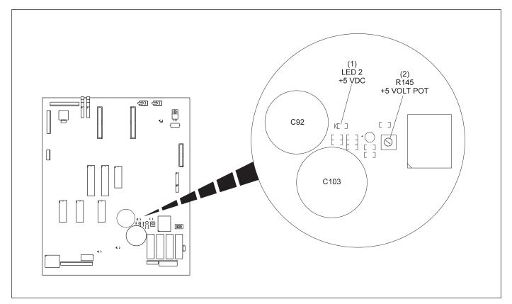
Figure 6-81. Adjusting +5VDC Potentiometer
