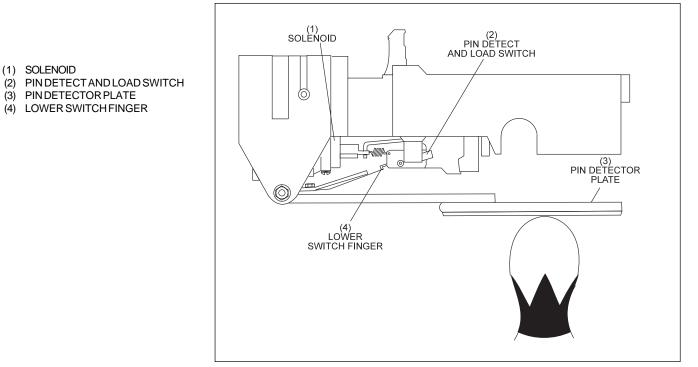
Figure 2-7. Pin Holder Detecting (GS-92)
