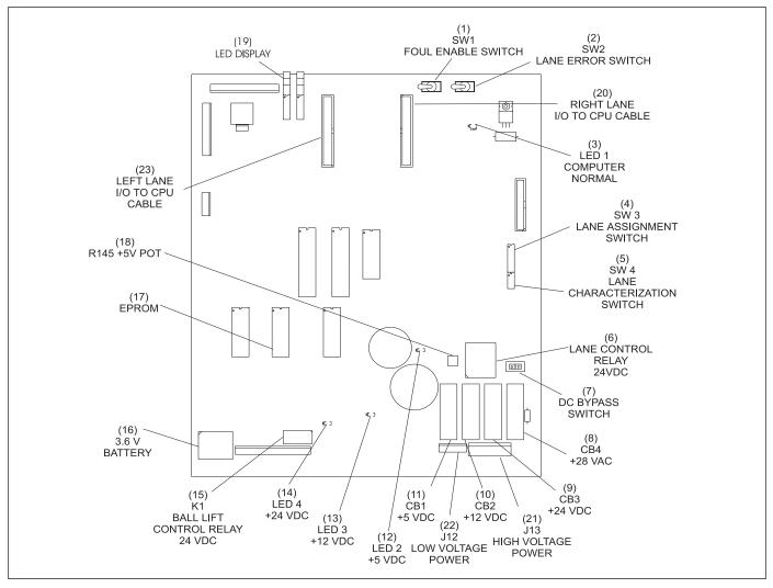
Figure 4-13. CPU PCB - Consolidated Low Voltage Control Box.
