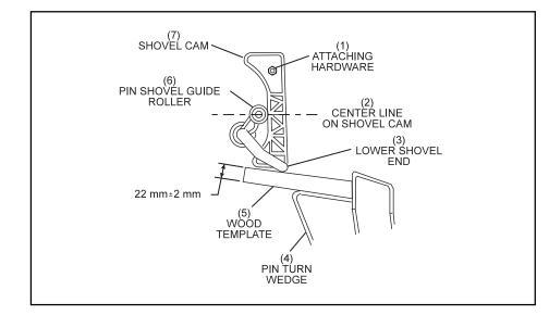
Figure 6-22. Elevator Pin Shovel Cam Adjustment.
