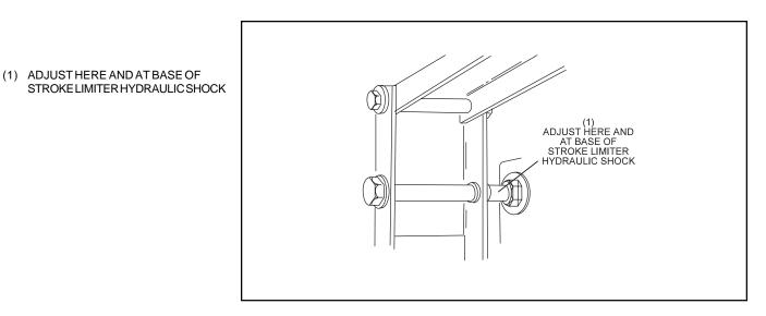
Figure 6-52. Stroke Limiter Centering Adjustment.
