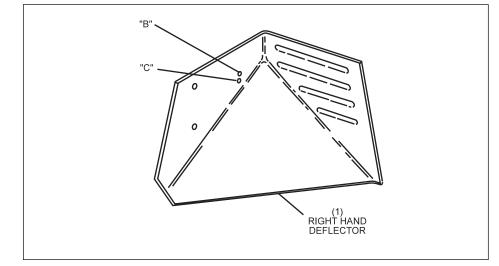
Figure 6-20. Right Hand Deflector Mounting Holes.
