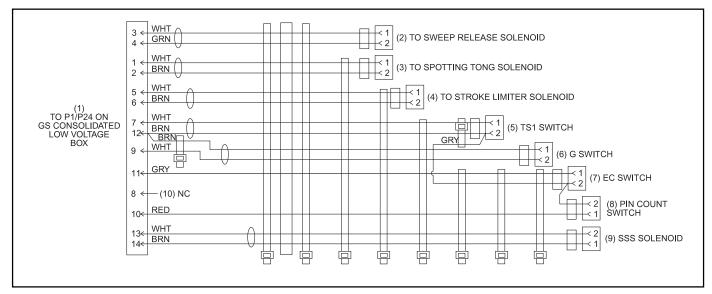
Figure 11-4. Left Side Function Cable (Part No. 47-142621-000)
