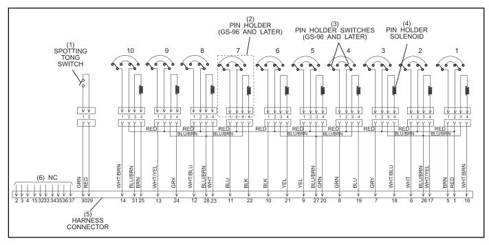
Figure 10-7. Schematic for Setting Table Harness Cable with Two Pinholder Switches (Part No. 47-243025-003)
