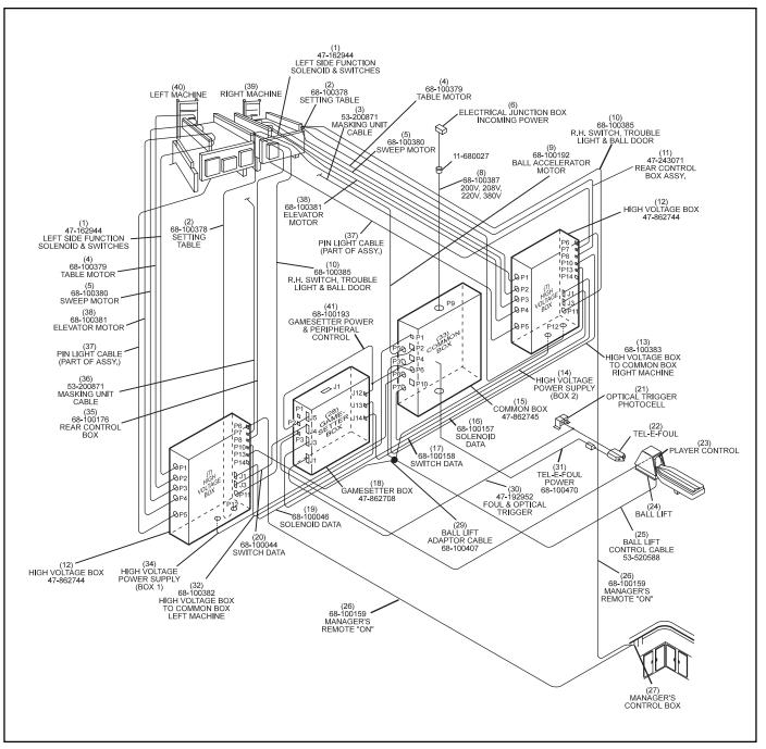
Figure 3-12. GS-Series Pinsetter with Universal Electronics.
