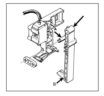
**14.** Front Distributor Shaft and Idler Gears Put a light film of grease on both gears.
