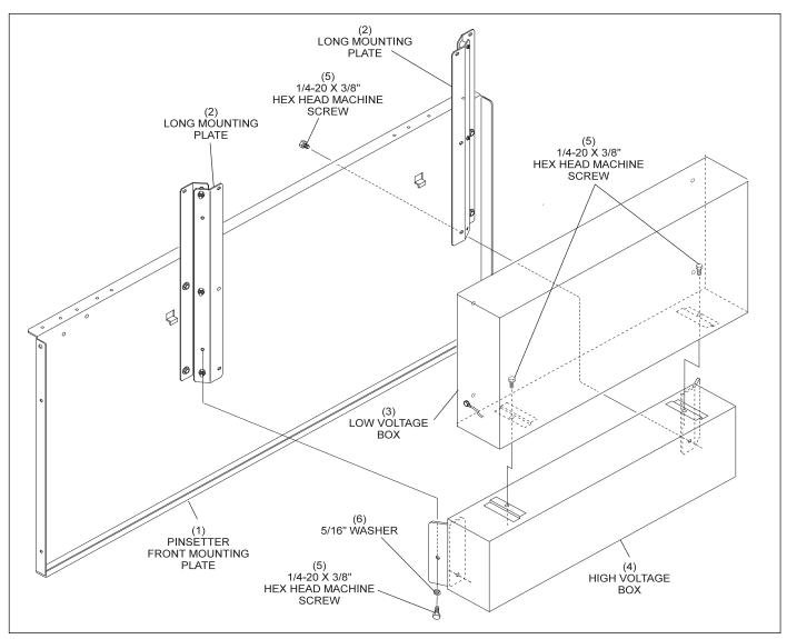
Figure 8-15. Consolidated High Voltage Box and Low Voltage Box Mounting Hardware.
