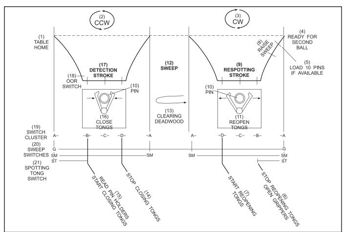
17. The pinsetter is ready for a second ball cycle.
