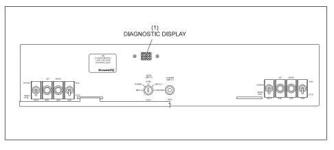
Figure 7-2. Top of Consolidated Low Voltage Box.
