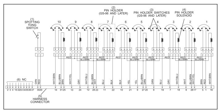
Figure 11-9. Schematic for Setting Table Harness with Two Pin Holder Switches (Part No. 47-243025-003)
