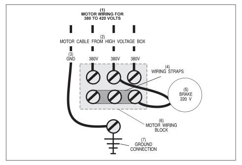
Figure 8-30. 380 Volt Motor Connection.
