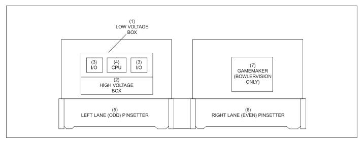
Figure 4-1. Electronic Control Box Layout (Consolidated Control System).
