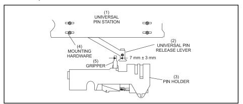
Figure 6-41. Universal Pin Release Lever.
