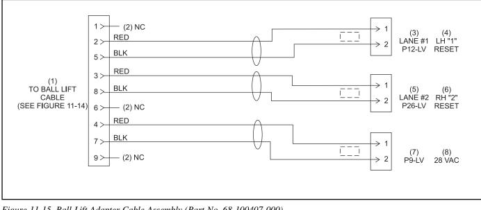
Figure 11-15. Ball Lift Adapter Cable Assembly (Part No. 68-100407-000)
