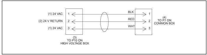
Figure 10-25. Remote "On" Left Lane Cable (Part No. 68-100382-000)
