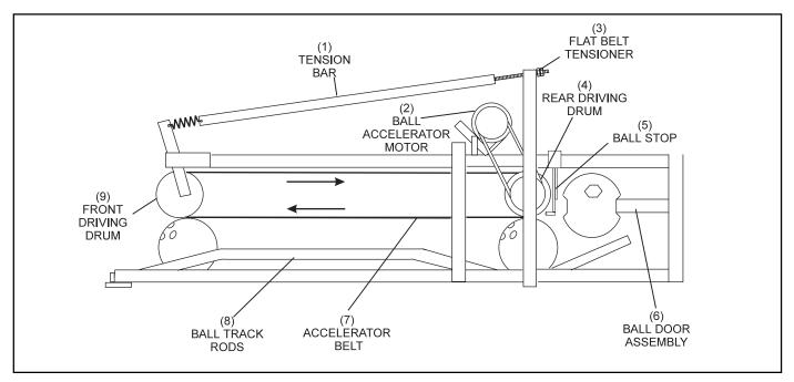
Figure 1-7. Ball Accelerator.
