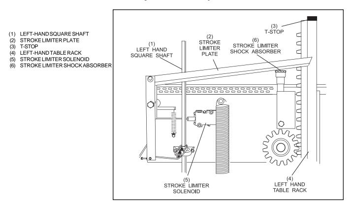
Figure 1-34. Stroke Limiter Assembly.
