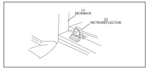
Figure 4-18. Retroreflector.
