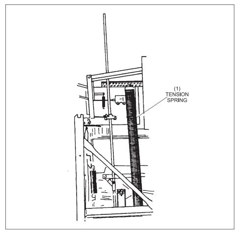
2. Remove the two tension springs from the setting table. Refer to *Figure* 8-3.
