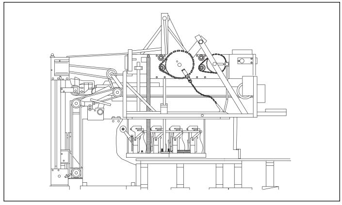
Figure 1-17. Setting New Pins.
