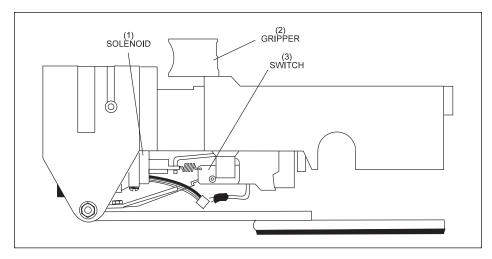
Figure 2-22. Pin Holder Horizontal - Up for Loading Pins.
