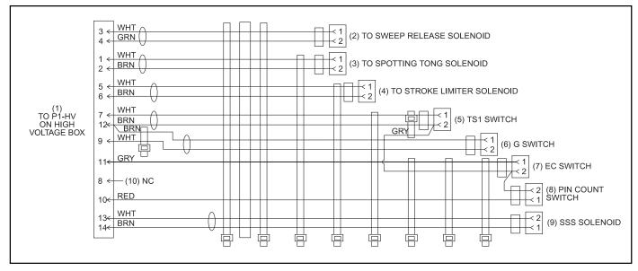
Figure 10-3. Left Side Function Cable (Part No. 47-162944-000)
