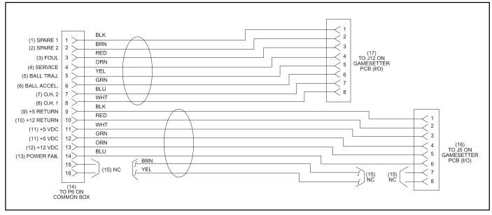
Figure 10-18. GS Power & Peripheral Control Cable (Part No. 68-100048-000)
