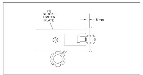
Figure 6-50. Stroke Limiter Clearance.
