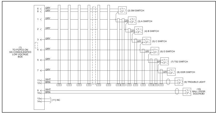
Figure 11-3. Right Side Function Cable (Part No. 47-142620-000)
