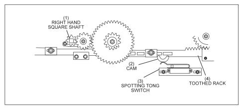
Figure 2-12. ST Switch with Tongs Open.
