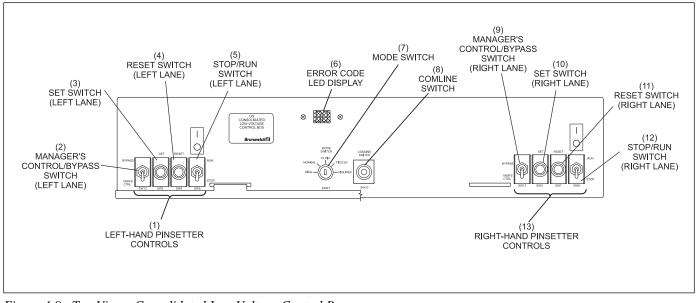
Figure 4-9. Top View - Consolidated Low Voltage Control Box.
