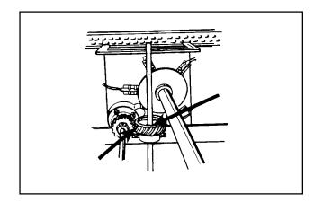
8. Spotting Tong Clutch Gear Cluster Grease the one or four gears lightly - DO NOT allow grease to get into the clutch mechanism.
