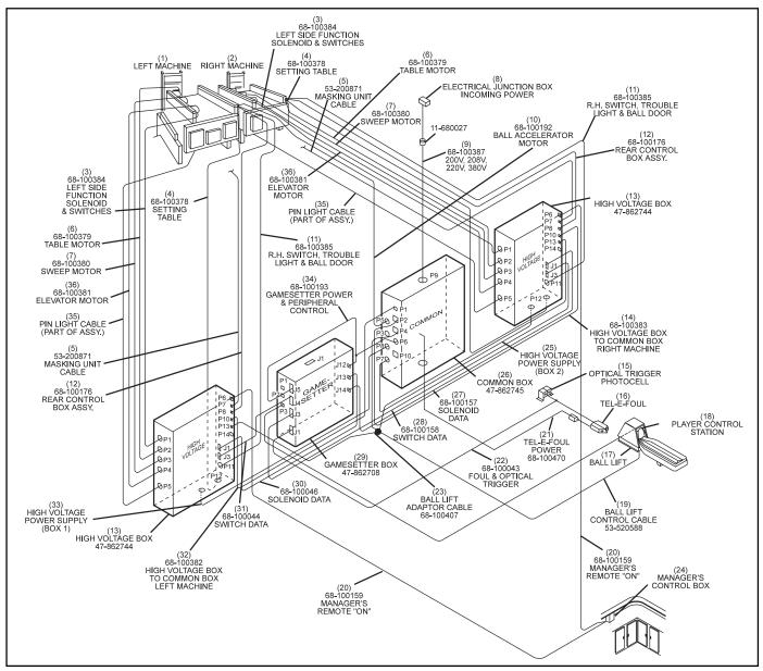
Figure 10-2. Universal Electronic Control System (Includes GS-92/96)
