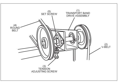
Figure 6-5. Tension Adjustment.
