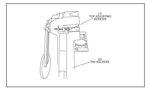
Figure 6-45. Adjusting an Individual Pin Holder.
