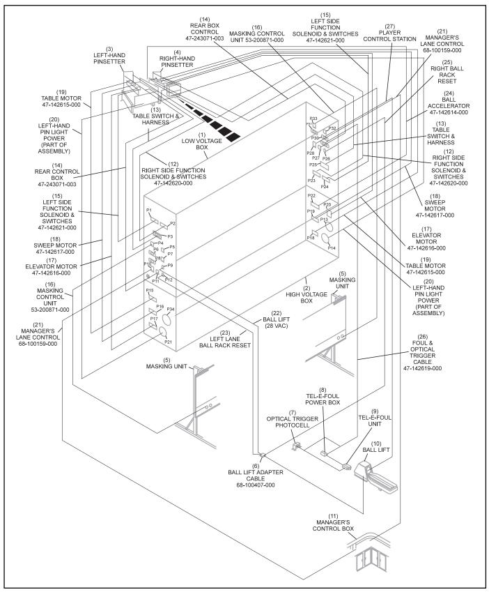
Figure 11-2. Consolidated Electronics Control System
