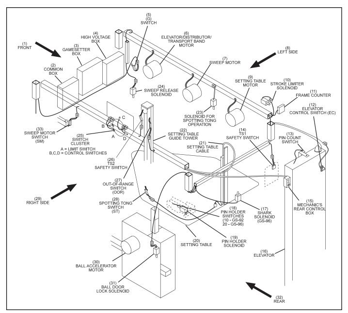
Figure 10-1. GS-92/96 Pinsetter Electrical System Overview with Universal Electronics
