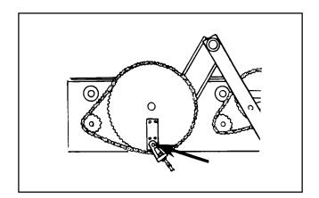
23. Stroke Limiter Plate's Bushings Apply one drop of oil to each of the four bushings
