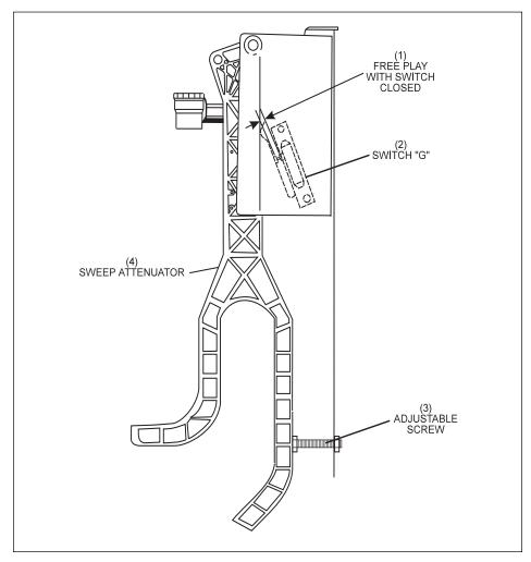
Figure 2-4. Attenuator Down, Closing "G" Switch.
