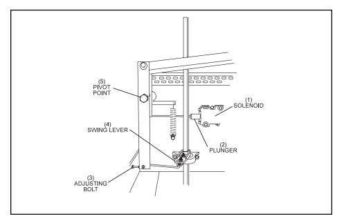
Figure 6-51. Stroke Limiter Adjustment.
