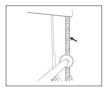
**3.** Elevator Chains Put a light coating of chain lubricant on both chains.
