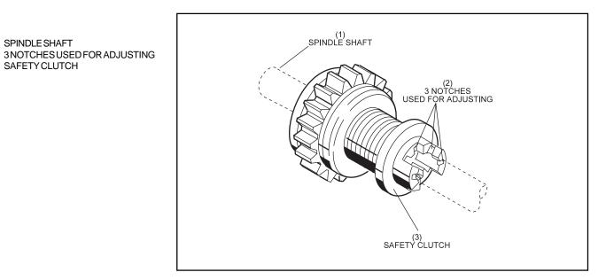
Figure 6-58. Spotting Tong Spindle Shaft Clutch.
