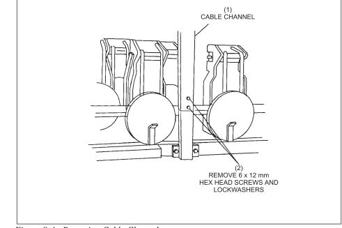
Figure 8-4. Removing Cable Channel.
