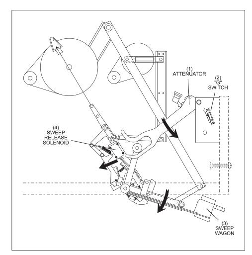
Figure 2-19. Sweep Release Solenoid.
