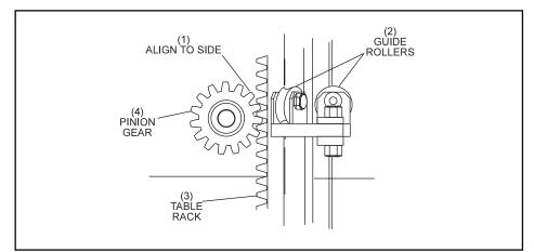
Figure 6-32. Table Rack Guide Rollers.
