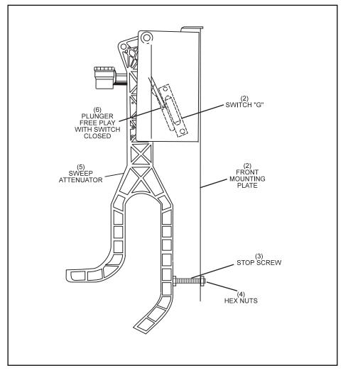
Figure 6-63. Sweep Attenuator/Switch "G" Adjustment.
