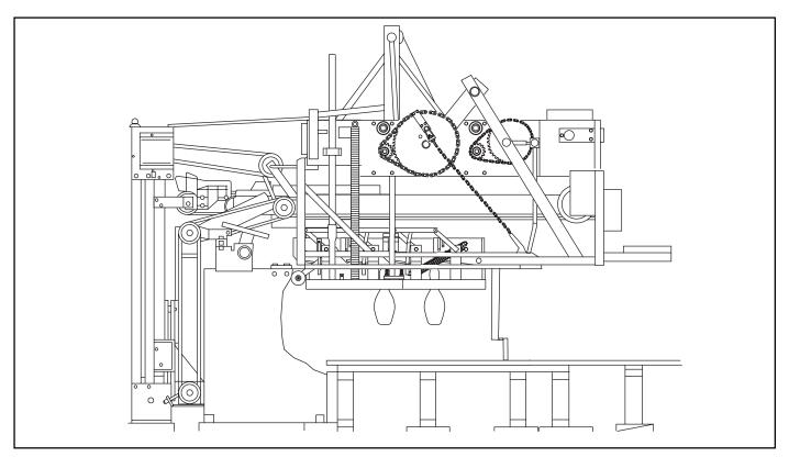
Figure 1-16. Spotting Tongs Closed - Picking Up Pins.
