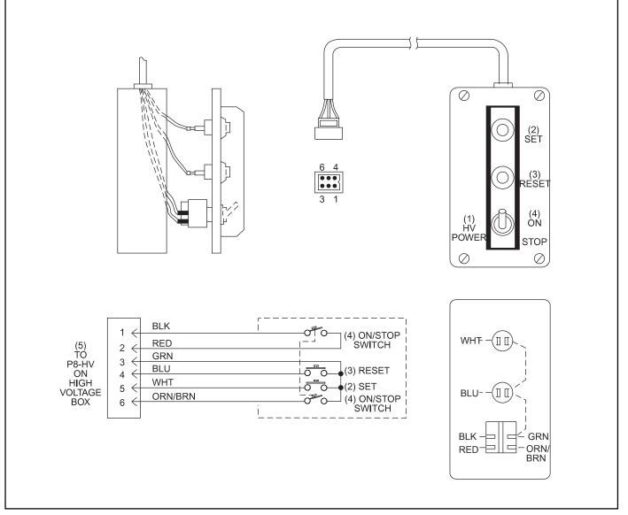
Figure 10-10. Rear Control Box Cable (Part No. 47-243071-003)
