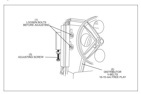
Figure 6-70. Adjusting Distributor V-Belts.
