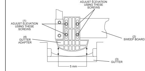
Figure 6-69. Sweep Board Gutter Adapter Adjustment.
