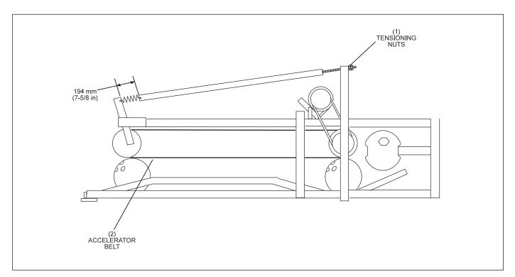
Figure 6-16. Ball Accelerator Flat Belt Tension Adjustment.
