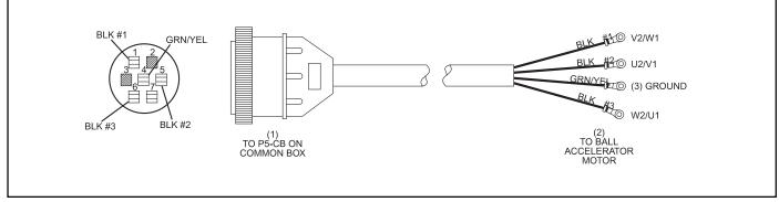
Figure 10-21. Ball Accelerator Cable (Part No. 68-100192-000)
