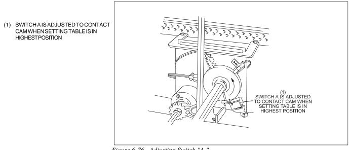
Figure 6-76. Adjusting Switch "A."
