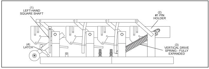
Figure 1-20. Table Up in Loading Pins Position.
