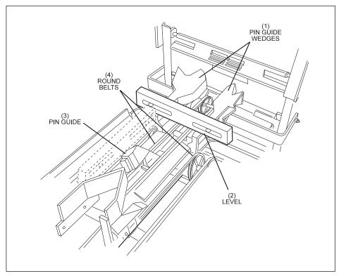
Figure 6-28. Shark Switch Leveling Adjustment - Side to Side.
