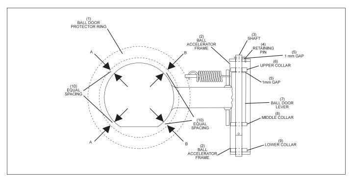
Figure 6-12. Ball Door Centering Adjustment.
