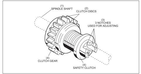
Figure 8-27. Reassembling Clutch.
