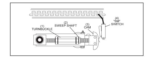
Figure 1-30. SM Switch Closed - Sweep Forward.
