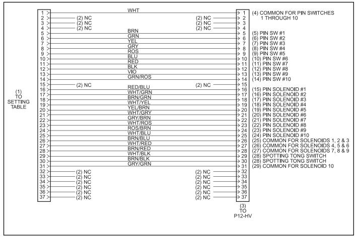
Figure 10-9. External Table Setting Cable (Part No. 68-100378-000)
