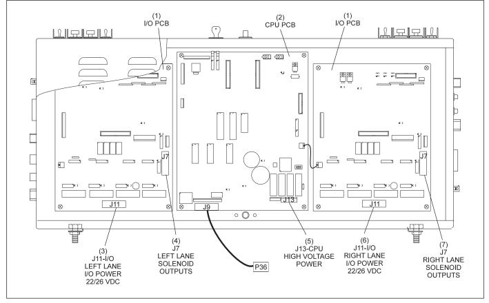
Figure 8-14. Internal View - Consolidated Low Voltage Control Box.
