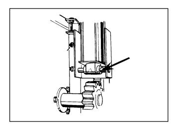
21. Sweep Wagon Connector Link Bearings Apply one drop of oil to the top and bottom bearing on each side.
