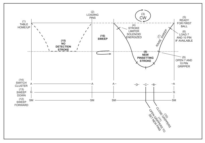
Figure 5-9. Second Ball Single Detect Cycle.
