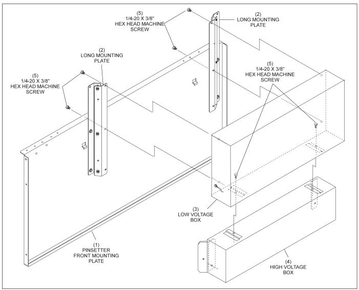
Figure 8-17. Consolidated High Voltage Box and Low Voltage Box Attaching Hardware.
