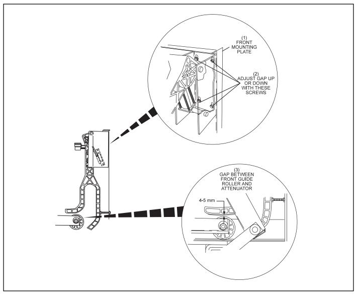
Figure 6-65. Gap Between Front Guide Roller and Attenuator.
