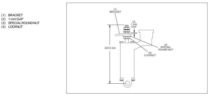
Figure 6-11. Adjust Jam Nuts on Shock Absorber Bracket.
