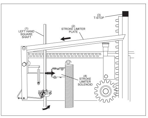
Figure 2-20. Stroke Limiter Solenoid.
