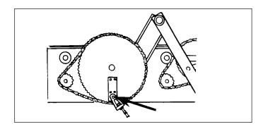
25. Sweep Release Chain ClevisA. Apply one drop of oil to the clevis's pivot point.
