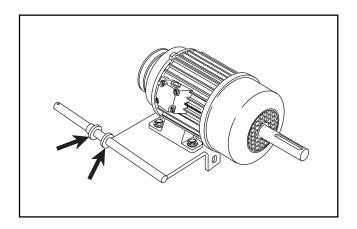
1. Motor Mounting Bracket Shafts Apply two drops of oil to each bushing on the shafts. This should be done for the table sweep, and distributor/accelerator motors.
