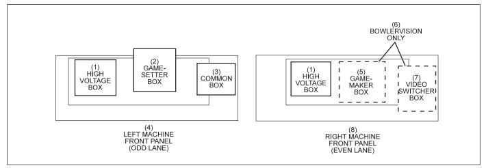
Figure 3-1. Electronic Control Box Layout.
