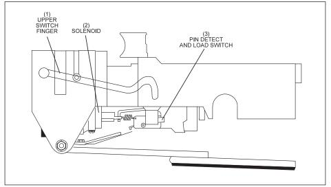
Figure 2-8. Pin Holder Loading (GS-92)
