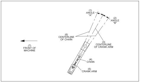
Figure 6-34. Crank Arm Angles.
