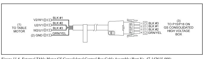
Figure 11-6. External TAble Motor GS Consolidated Control Box Cable Assembly (Part No. 47-142615-000)
