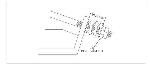
Figure 6-3. Transport Band Tension Using Compression Springs.
