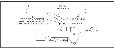
Figure 6-40. Pin Release Lever.
