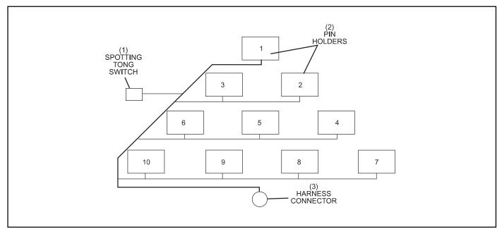
Figure 10-8. Pictorial of Setting Table Harness Cable (Part No. 47-243025-003)
