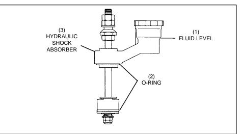
Figure 9-1. Hydraulic Fluid Level.
