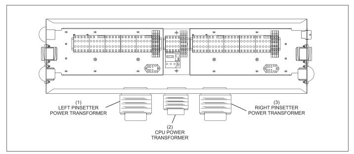
Figure 4-5. Consolidated High Voltage Box Transformers.
