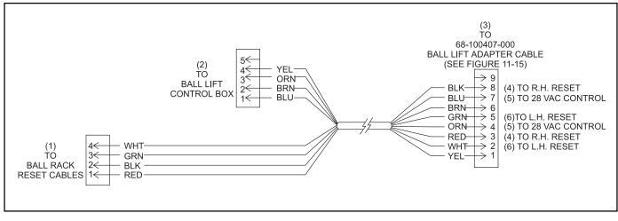
Figure 11-14. Ball Rack Lane Cable Assembly (Part No. 53-520588-000)
