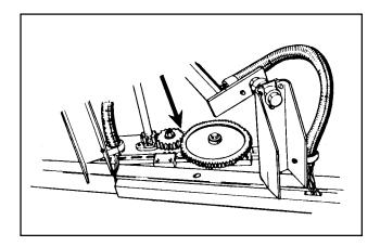
**11. Ball Cushion Bushings** Grease both sides as required.
