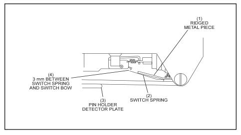
Figure 6-53. Pin Holder Switch Adjustment.
