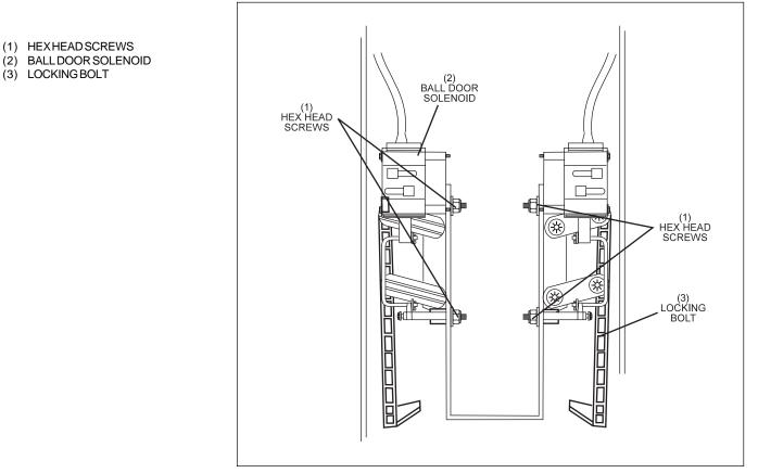
Figure 6-14. Ball Door Solenoid.
