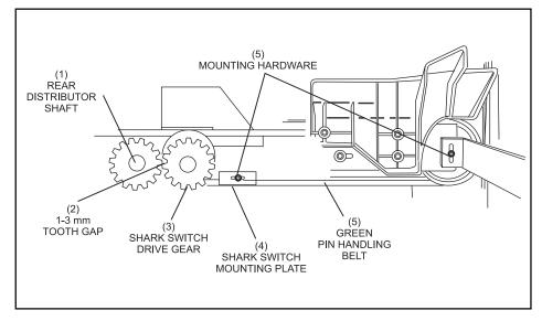
Figure 6-26. Clearance Between Drive Gear and Spur Gear
