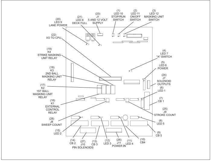
Figure 4-11. I/O PCB - Consolidated Low Voltage Control Box.
