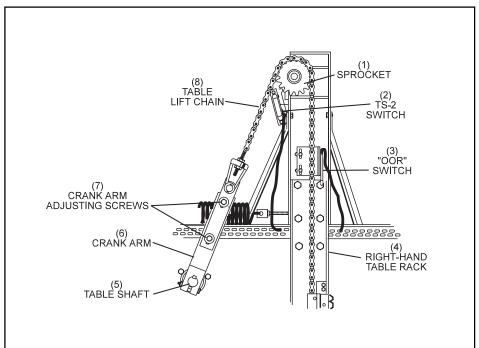
Figure 1-36. Right-Hand Guide Tower Assembly.
