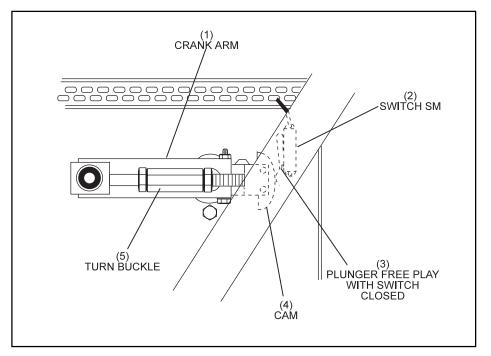
Figure 6-62. Sweep Motor Switch "SM" Adjustment.
