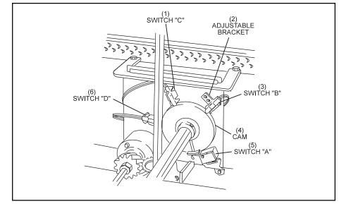
Figure 6-55. "B" Switch Adjustment.
