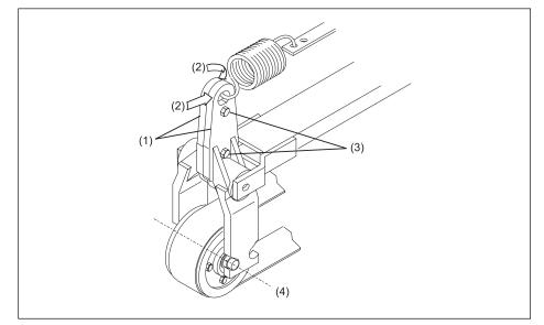
Figure 6-17. Loosen Hardware Securing Pivot Levers
