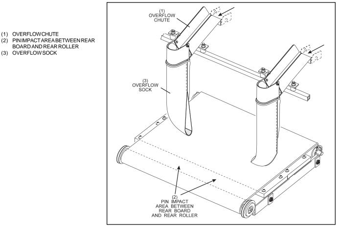
Figure 1-14. Pin Overflow Area.
