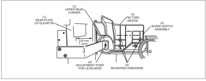
Figure 6-27. Pin Turn Wedge Positioning.
