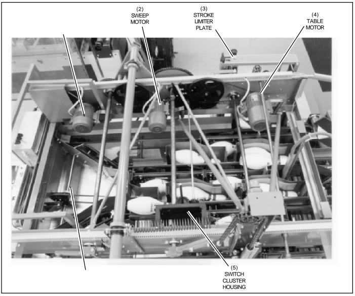
Figure 1-33. Drive Frame Assemblies.
