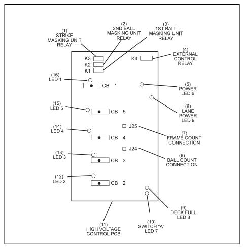
Figure 3-7. Universal High Voltage Control PCB.
