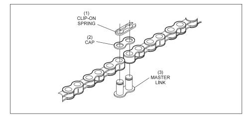
Figure 8-33. Chain Repair.
