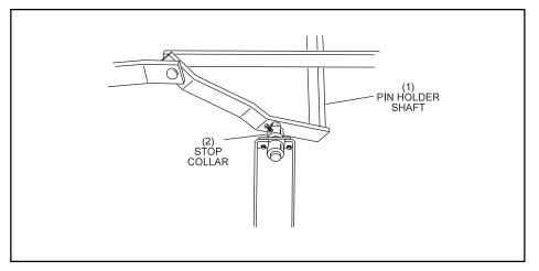
Figure 6-43. Adjusting an Entire Row of Pin Holders.
