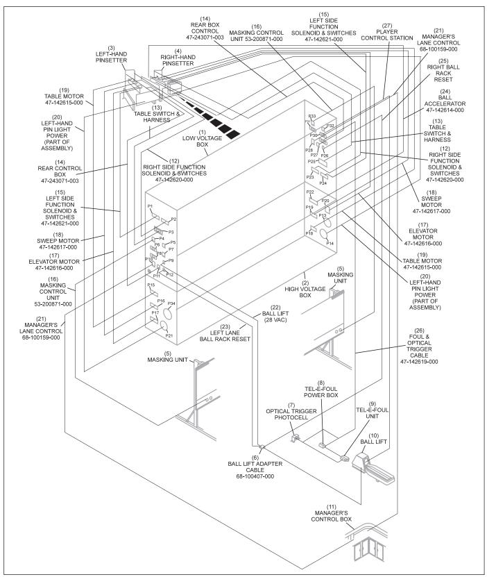
Figure 8-12. Consolidated Voltage Cable Connections and Routing.
