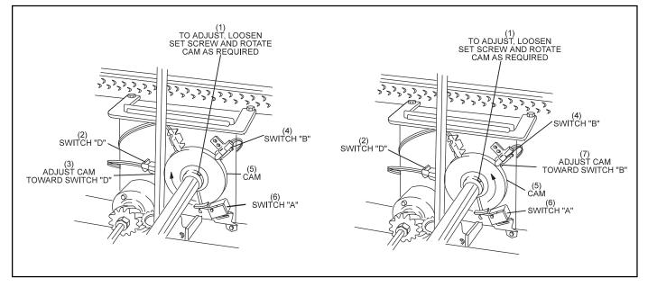
Figure 6-35. Adjusting Angles "A" and "B."
