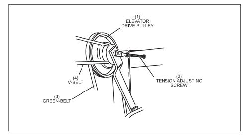
Figure 6-23. Tension Adjustment.
