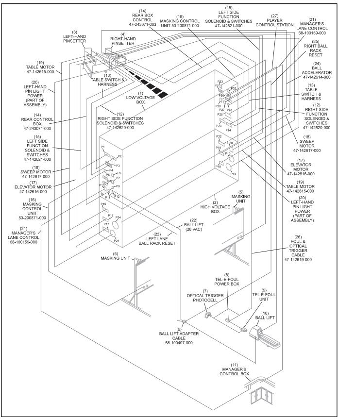
Figure 4-16. GS-Series Pinsetters with Consolidated Electronics.
