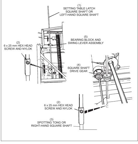
Figure 8-5. Disconnecting Square Shafts.
