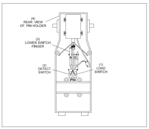
Figure 2-9 Pin Holder Switches (GS-96 and Early GS-98).
