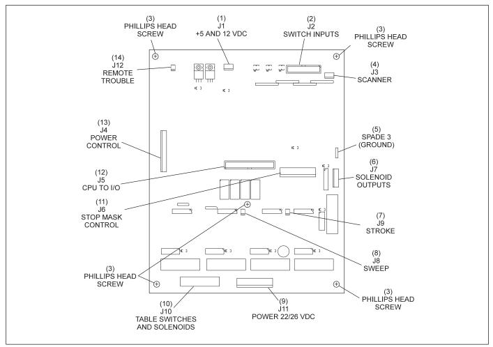
Figure 8-18. Consolidated Low Voltage Box I/O PCB Removal.
