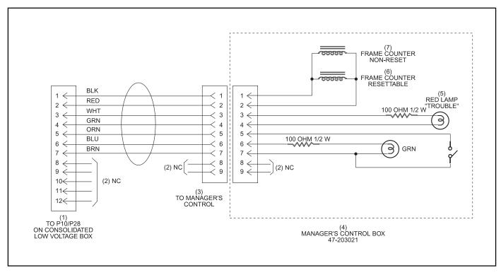
Figure 11-16. Manager's Remote Control Cable Assembly (Part No. 68-100159-000)
