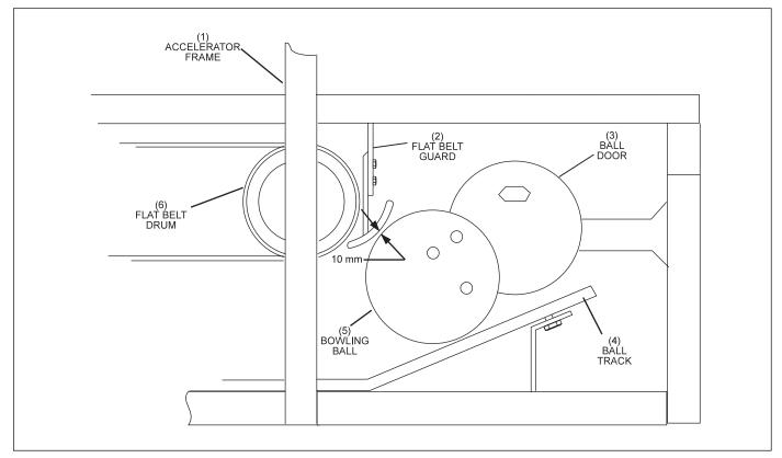
Figure 6-15. Ball Accelerator Flat Belt Guard Adjustment.
