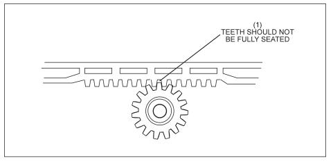
Figure 6-74. Adjusting for Proper Tooth Gap.
