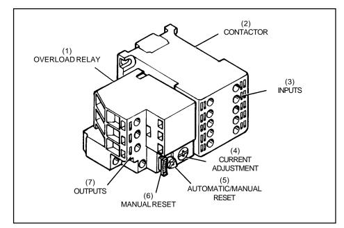
Figure 3-6. Motor Contactor and Relay.
