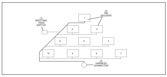
Figure 11-10. Pictorial for Setting Table Harness (Part No. 47-243025-003)
