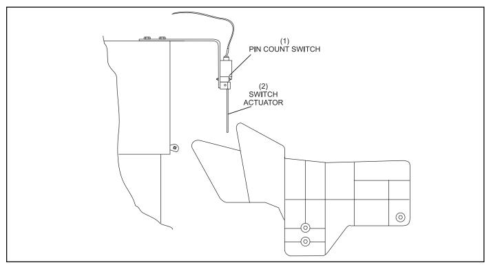
Figure 1-12. Pin Count Switch and Shark Solenoid (GS-96s and Later)
