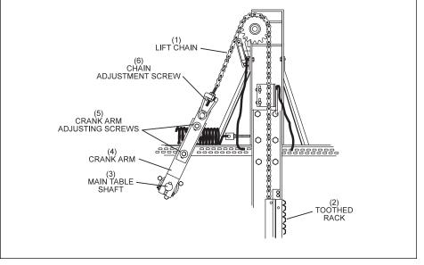
Figure 6-37. Table in Lowest Position (Universal Pin Station).
