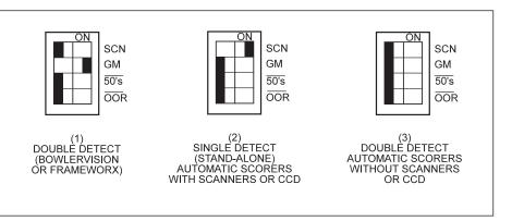
Figure 8-11. Characterization Switch Positions
