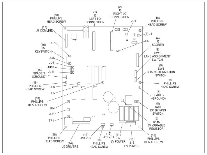
Figure 8-19. Consolidated Low Voltage Box CPU PCB Removal.
