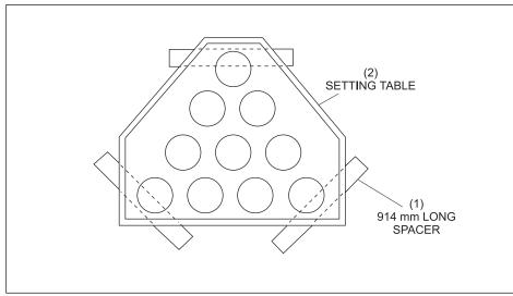
Figure 8-2. Placing Spacers.
