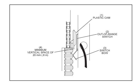
Figure 6-60. Table Rack Cam and Switch.
