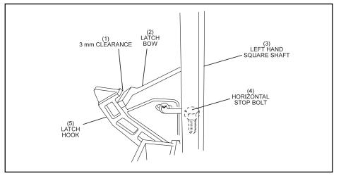
Figure 6-56. Rear Swing Shaft's Latch Bow and Latch Hook.
