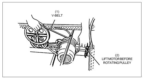
Figure 8-1. Manually Raising or Lowering the Setting Table.
