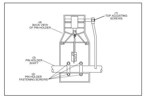
Figure 6-44. Adjusting an Individual Pin Holder.
