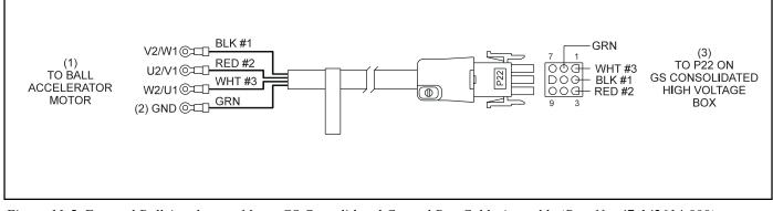
Figure 11-5. External Ball Accelerator Motor GS Consolidated Control Box Cable Assembly (Part No. 47-142614-000)
