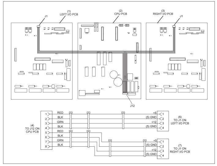
Figure 6-80. Checking Voltage on the I/O PCB
