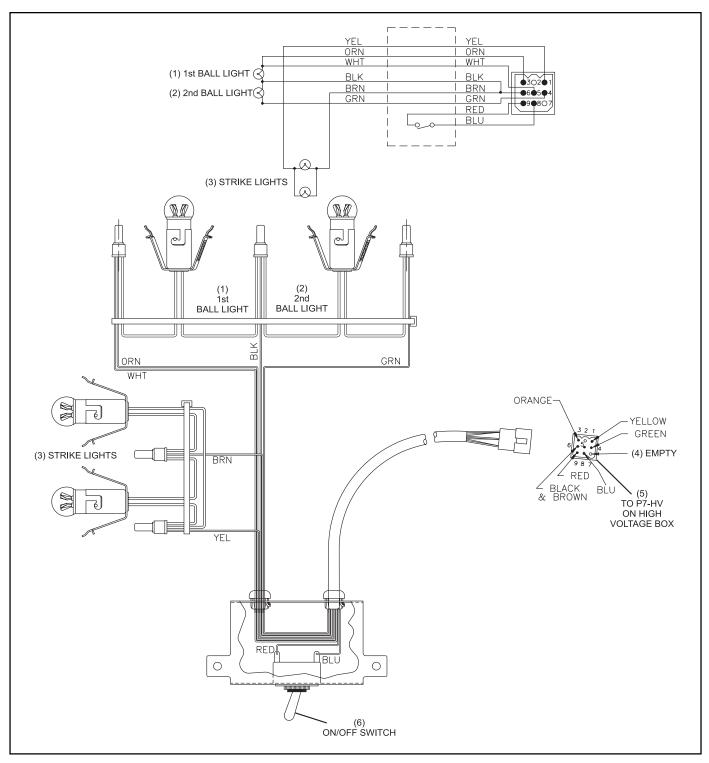
Figure 11-13. Masking Unit Cable Assembly (Part No. 53-200871-000)
