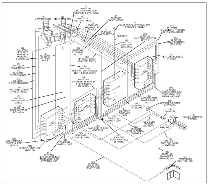
Figure 8-7. Universal Voltage Cable Connections and Routing.
