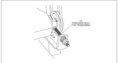
Figure 6-4. Jam Nut for Tensioning the Transport Band.
