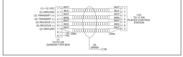
Figure 10-19. Player Control Station Cable (Part No. 68-100050-000)
