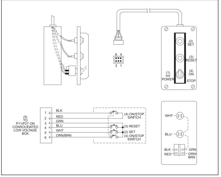
Figure 11-11. Rear Control Box Cable Assembly (Part No. 47-243071-003)
