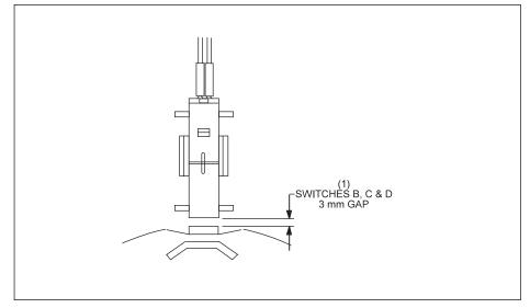
Figure 6-75. Adjusting Table Position Switches.
