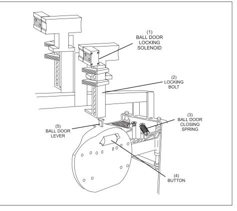
Figure 2-18. Ball Door Solenoid.
