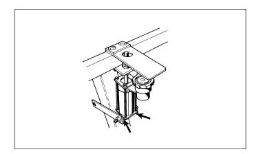
12. Hydraulic Shock Absorber BushingA. One drop of oil each side of the bushing.
