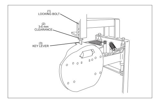
Figure 6-13. Adjusting Locking Bolt.
