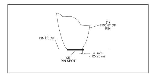
Figure 6-42. Proper Pin Position.
