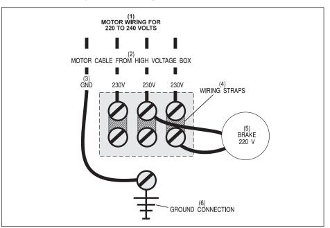
Figure 8-29. 230 Volt Motor Connection.
