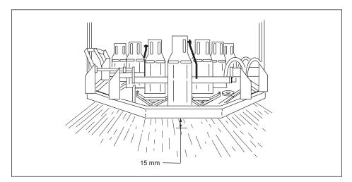
Figure 6-38. Checking Table's Lowest Position.
