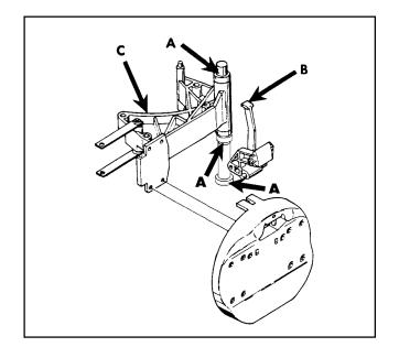
1. Pin Shovel Shafts One drop of oil on each pivot point.
