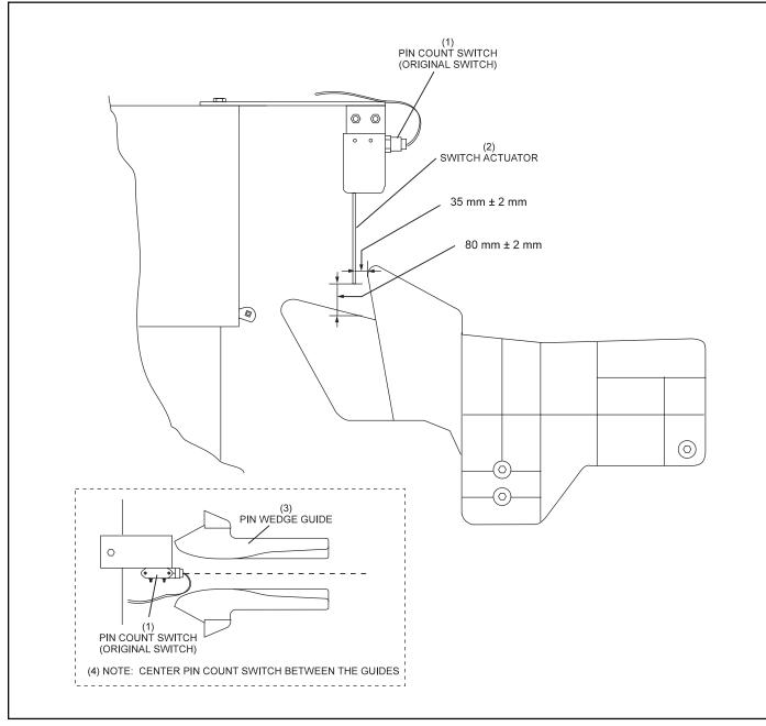
Figure 6-24. Original Style Pin Count Switch
