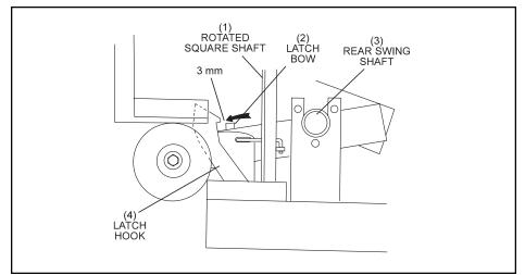
Figure 6-57. Adjusting Swing Lever.
