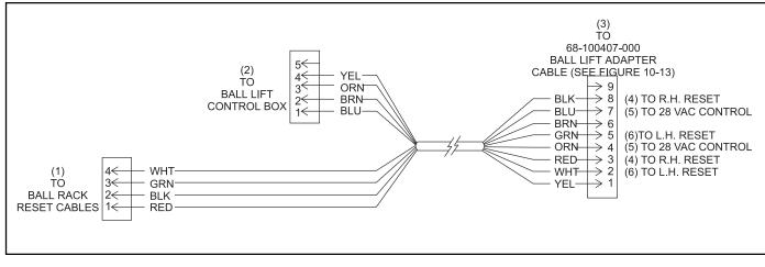
Figure 10-12. Ball Rack Lane Cable (Part No. 53-520588-000)
