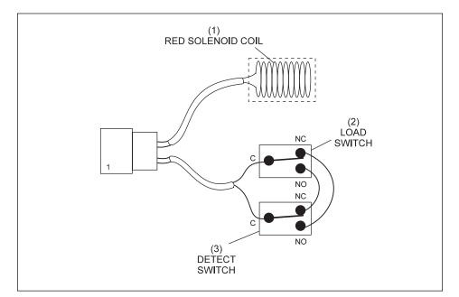
Figure 2-11. Pin Holder Wiring
