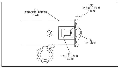
Figure 6-49. Stroke Limiter Plate.
