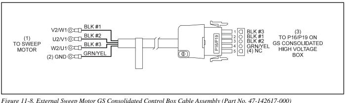
Figure 11-8. External Sweep Motor GS Consolidated Control Box Cable Assembly (Part No. 47-142617-000)
