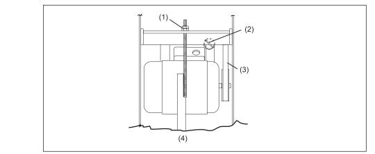
Figure 6-18. Loosen Jam Nuts
