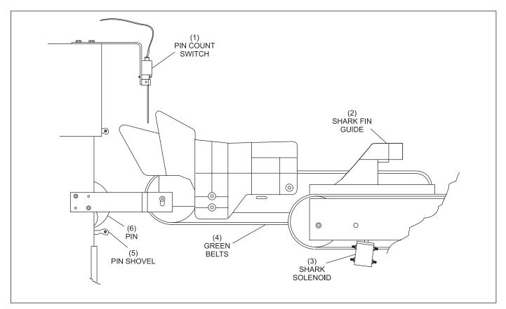
Figure 2-16. Pin Count Switch and Shark Solenoid (GS-96s and Later)
