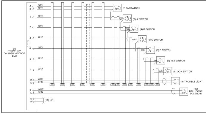
Figure 10-4. Right Side Function Cable (Part No. 68-100385-000)
