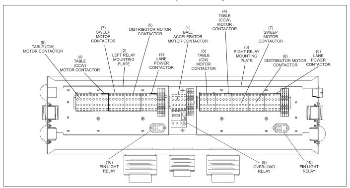
Figure 4-6. Internal View - Consolidated High Voltage Control Box.
