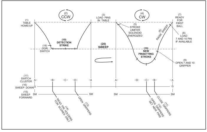
Figure 5-10. Second Ball Double Detect Cycle.
