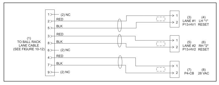
Figure 10-13. Ball Lift Adapter Cable (Part No. 68-100407-000)
