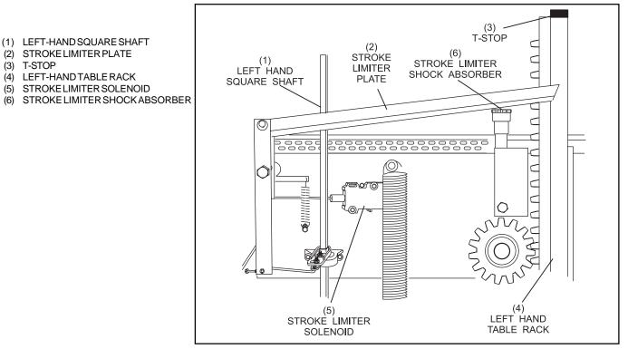
Figure 1-27. Left-Hand Table Rack with "T" Stop.
