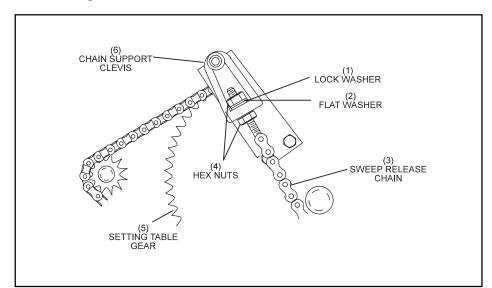
Figure 6-68. Sweep Board Height Adjustment.
