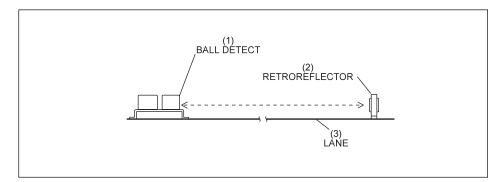
Figure 6-1. Ball Detect and Retroreflector.
