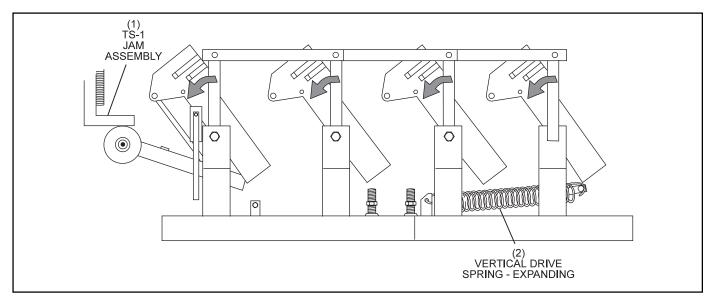
Figure 1-22. Table Raising - Pin Holders Returning to Horizontal Position.
