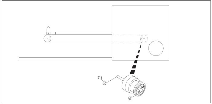
Figure 6-19. Remove Shaft Ends.
