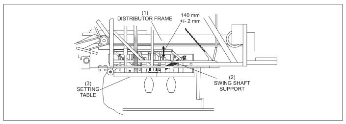
Figure 6-36. Raised Position Measurement.
