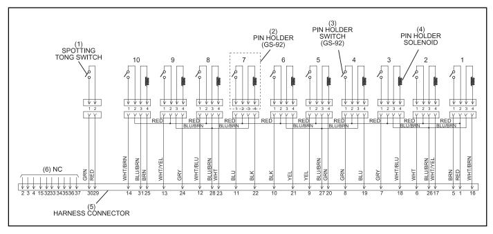
Figure 10-6. Schematic for Setting Table Harness Cable with One Pinholder Switch (Part No. 47-243025-003)
