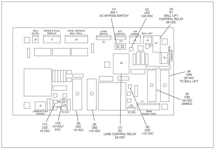
Figure 3-4. Universal Common Box PCB.
