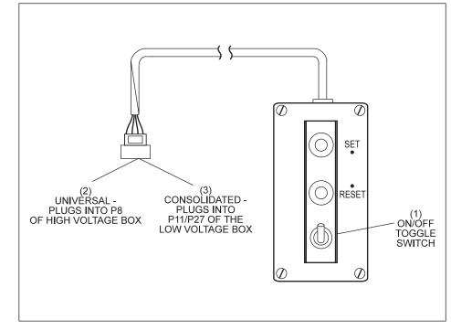
Figure 2-5. Mechanic's Rear Control Box.
