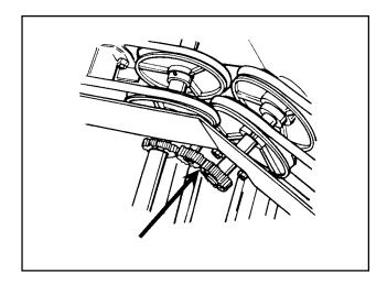
**4. Setting Table Pinion Gears** Entire chain needs a light coating of chain lubricant.
